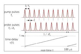
The TL-1000-ASOPS controls the time delay between pump and probe pulses by slightly differing repetition rates ( $f_R \sim 1$  GHz). The difference in  $\Delta f_R$  determines the scan rate, while the measurement window is given by the inverse of the repetition rate I/ $f_R$ =1ns. Here,  $\Delta f_R$  is 10 kHz, i.e. the time-delay is repetitively ramped with a 100  $\mu$ s period.
