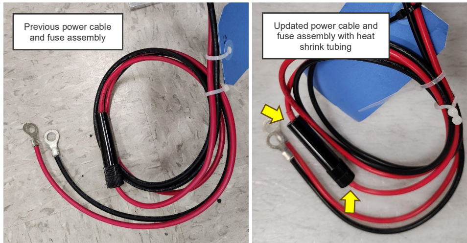
Figure 1. Previous power cable and fuse assembly is shown on the left, and the updated power cable and fuse assembly is shown on the right.
