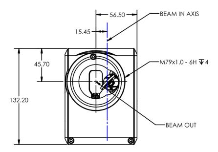
Figure 3: Dimensions of "top I/O"- and "side I/O"-variant in millimeters
