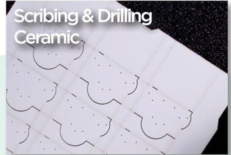
The high peak power is essential to minimizing heat build-up and avoid cracking when processing brittle materials such as alumina, ceramic and quartz glass. Excellent beam quality allows for very small features and clean symmetric holes.
