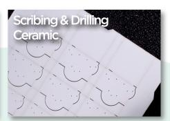
The high peak power is essential to minimizing heat build-up and avoid cracking when processing brittle materials such as alumina, ceramic and quartz glass. Excellent beam quality allows for very small features and clean symmetric holes.
