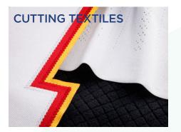
When cutting many natural and synthetic textiles cut edge charring or melting is caused by excessive heat build-up in the material. High peak power and fast pulse rise time eliminates this issue, expanding the range of materials for laser processing.
