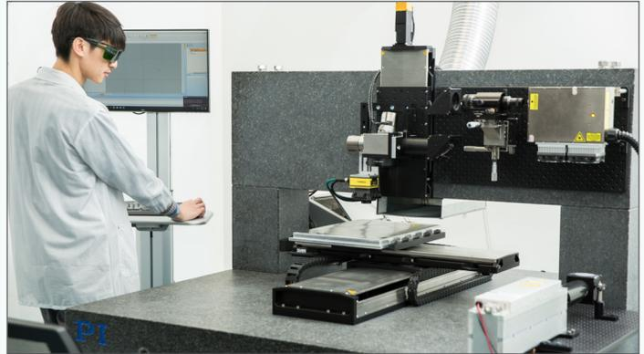
SyncMaster – advanced laser scanning head and XY linear stage synchronization expands work field size and fits production environments with unmatched accuracy and speed.
