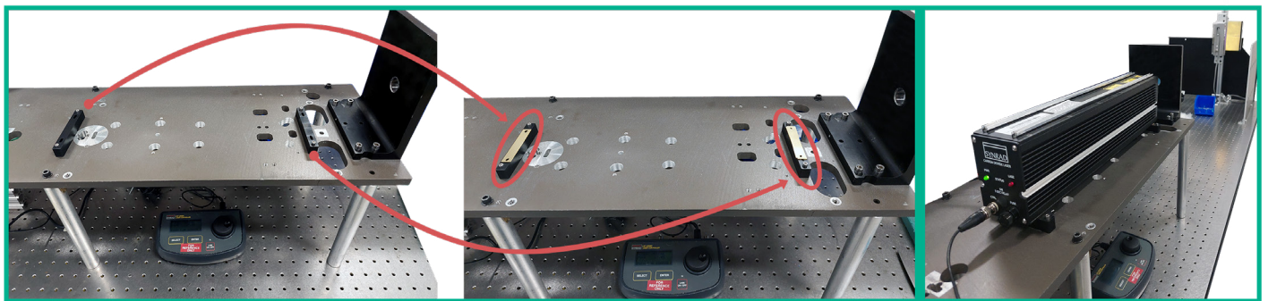
Fig 5. Assembling shims on to the mounting feet (left) before laser is mounted (right).
