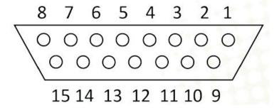
The external Interlock will disable the system (laser emission with cease) whenever the circuit is open. The status window on the LCD screen will read 'DISABLED: KEYSWITCH/INTLK'. To re-enable the laser the Interlock circuit must be closed and then the "Switching On" instructions followed (Section 5.).
