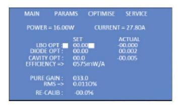
By rotating the jog wheel, position the cursor over the LBO OPT and press the 'down' button. This will select the SET value for LBO OPT, as indicated by the modify cursor (shown above)
