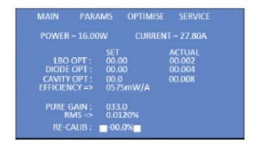
All the factory settings are not affected when the new off-sets are stored in the memory. To return to the factory settings simply return each of the parameters to zero SET value.
