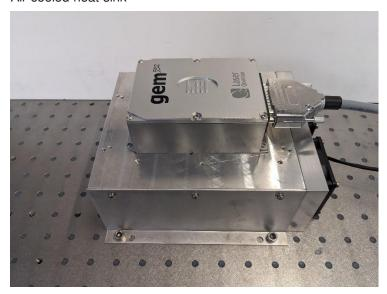
If the **finesse pure** is not attached to an adequate heatsink or cooling solution or the **fpu60** cooling intakes are blocked, then these components will gradually increase in temperature.
