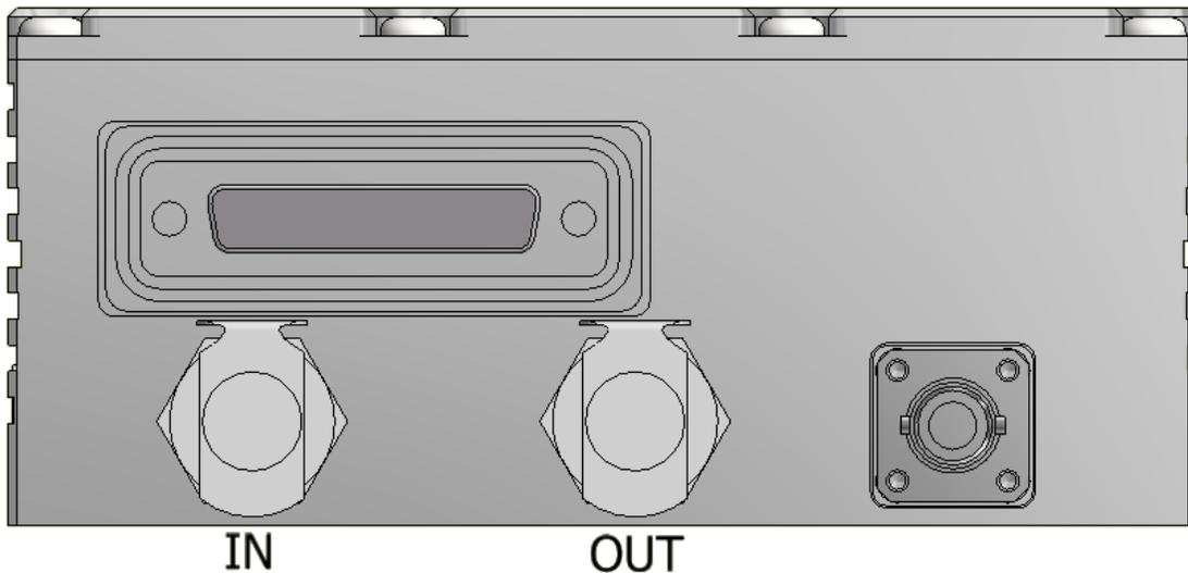
The required water connectors are standard CPC coupling inserts and a tubing size of approximately 1/4" or 3/8" is suitable. For further information on heatsinking your laser system, please consult your sales representative who may be able to provide an alternative heatsink solution if water cooling is not possible.
