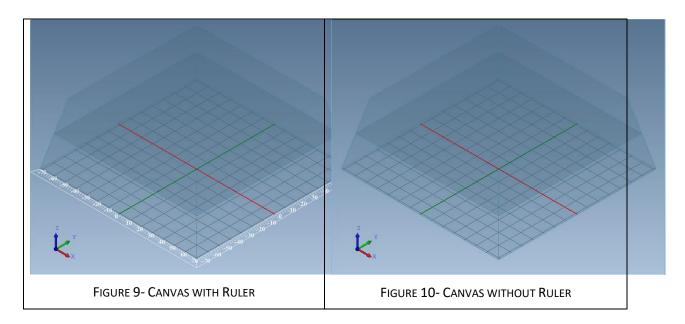
A ruler is displayed along the **X** and **Y** axis of the drawing canvas in order to help you adjust the position of the 3D model in the drawing canvas.
