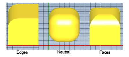
FIGURE 50- FILLETS ON DIFFERENT SELECTION MODES
