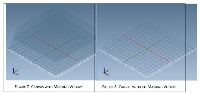
Any 3D models or sections of 3D models which are placed beyond the marking volume will not be marked by the scan head.
