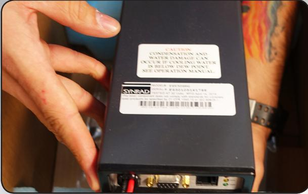
**6.1** Handling the laser by the **base plate** to carry the laser without risk of knocking it out of alignment.
