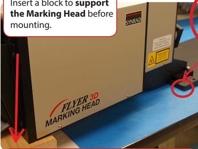
**7.1** Place the Marking Head on the rail as shown, a block may be used to support the marking head until it is mounted to the rail.
