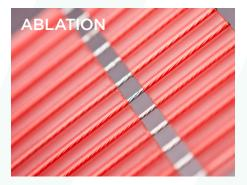
Optimized wavelengths and excellent poser stability allow precise removal of insulation and coatings without damaging the underlying materials.
