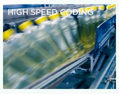
Easily applies permanent alpha numeric codes, bar codes, text, and expiration dates to a variety of packaging materials that will not smear or rub off
