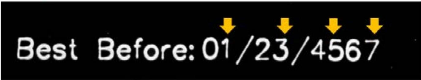
Each mark uses the same parameters: Marking Speed: 15 m/s; Jump Speed: 30 m/s; Mark Delay: 60  $\mu$ s; Jump Delay: 100  $\mu$ s, and Poly Delay: 60  $\mu$ s. Note that with VPD enabled, corners are less sharp, but throughput was increased by 12%.
