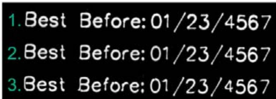
The second is a MOVIA and fiber laser system marking coated glass to show achievable character formation at various speeds
