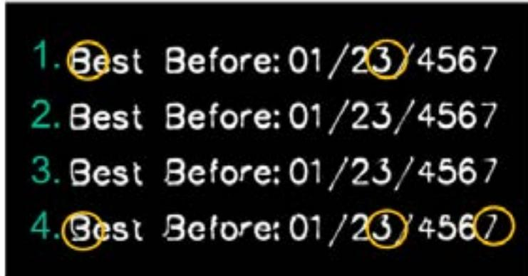
Poly Delay: delay inserted between two marking segments that ensures sharper corner formation. If this delay is too short, characters will appear misshapen. Too long of a delay will increase processing time and could cause burn-ins at the corners
