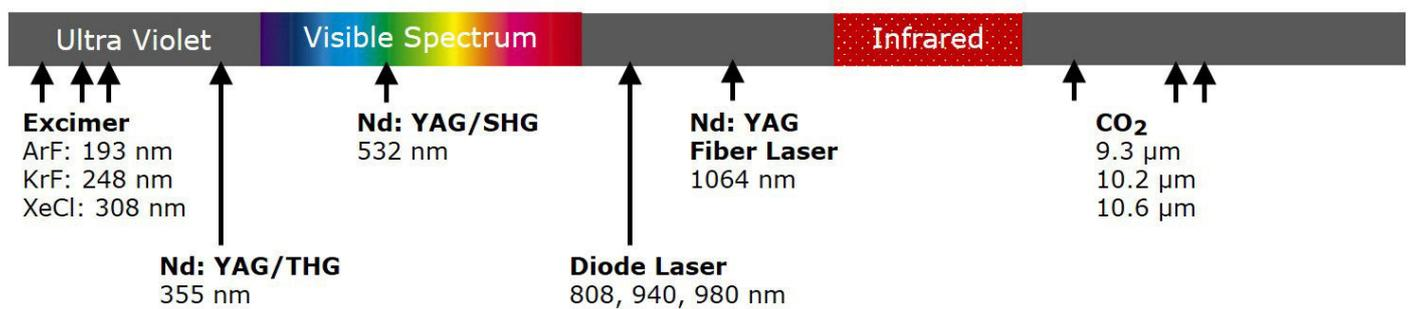
CO<sub>2</sub> lasers have long wavelengths, around 9.3 – 10.6 μm, with 10.6 μm as the most common. These wavelengths pair nicely with the absorption spectrum from polymers, ceramics, textiles, natural materials like paper or wood, and certain metals. By contrast, the shorter wavelength YAG or Fiber lasers tend to have better absorption in metals.
