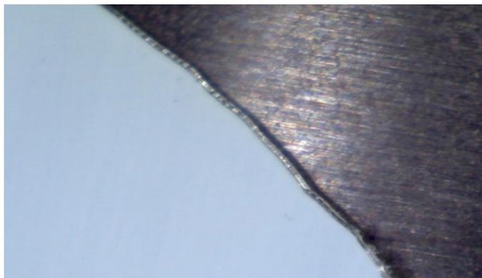
10.2 μm: Cutting is 2.5X faster, and produces a crisp edge with minimal melt lip.
