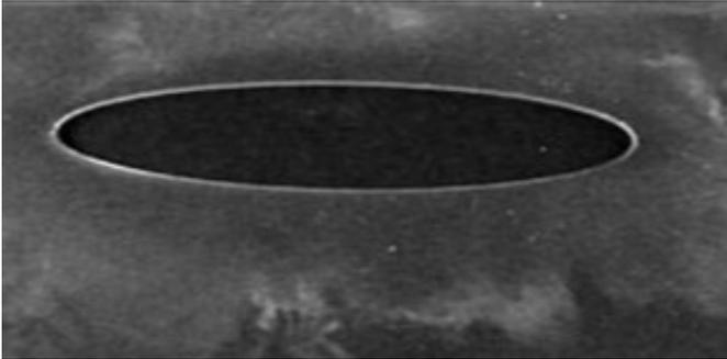
9.3  $\mu\text{m}$ : Cutting produces a clean edge with no residue and minimal melting.
