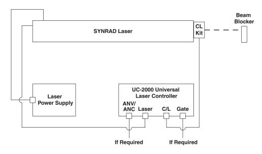
Figure A-1 Typical closed loop setup
