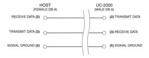
Figure 3-6 RS-232 cable wiring diagram
