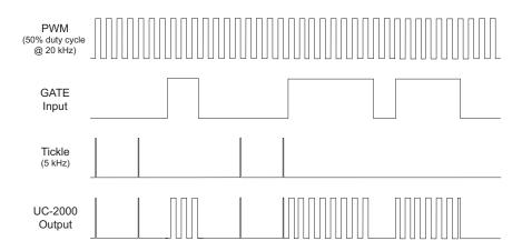
Figure 3-4 UC-2000 input/output signal relationships
