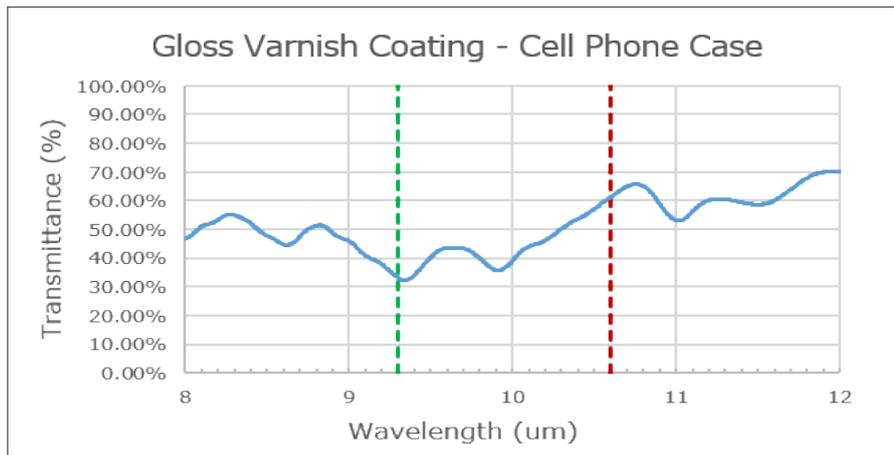
The transmission curve indicated that a laser at 9.3  $\mu\text{m}$  had 25% less transmission than the more common 10.6  $\mu\text{m}$  lasers available. The lower transmission rate would enable Novanta's Synrad laser to lightly mark the gloss coating at high speed while avoiding any damage to the underlying base plastic.
