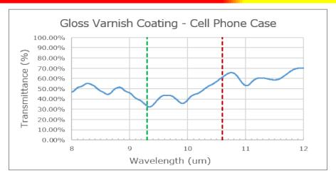
The transmission curve indicated that a laser at 9.3  $\mu$ m had 25% less transmission than the more common 10.6  $\mu$ m lasers available. The lower transmission rate would enable Novanta's Synrad laser to lightly mark the gloss coating at high speed while avoiding any damage to the underlying base plastic.
