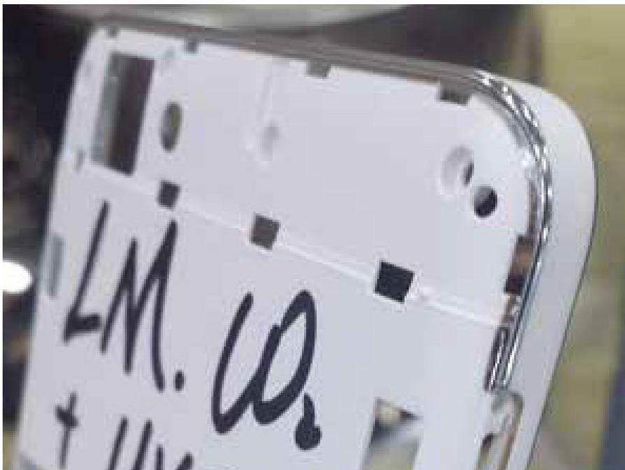
Matching the quality appearance of a metal cell phone case with a plastic case required two different finishes, a highly polished “chrome-like” edge and a brushed satin finish for the flat surfaces. The plastic cell phone frames had a glaze coating and Novanta Application Engineers determined that impacting the gloss coating without affecting the underlying base plastic both increases the metallic appearance of the mark and provides better durability.
