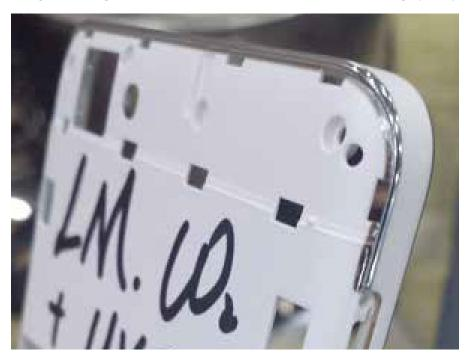
Matching the quality appearance of a metal cell phone case with a plastic case required two different finishes, a highly polished "chrome-like" edge and a brushed satin finish for the flat surfaces. The plastic cell phone frames had a glaze coating and Novanta Application Engineers determined that impacting the gloss coating without affecting the underlying base plastic both increases the metallic appearance of the mark and provides better durability.
