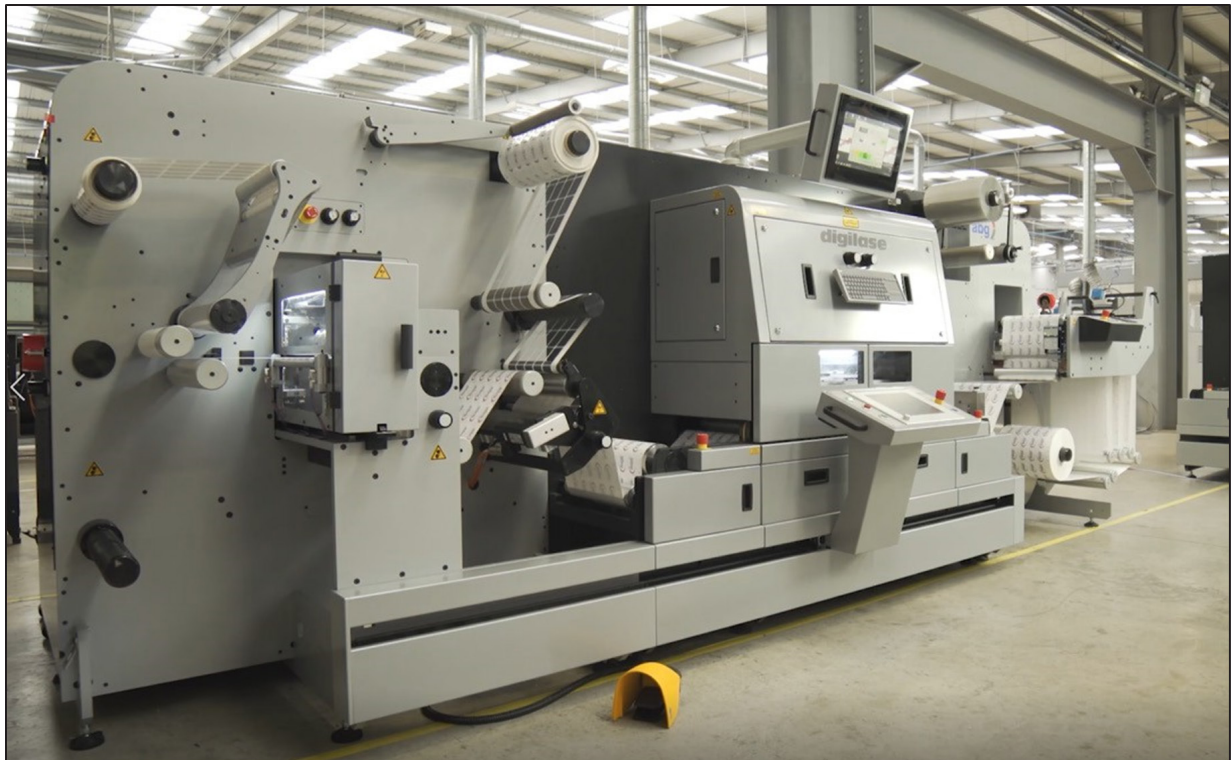
Fig. 3: Example of a roll-to-roll label cutting system. The scan head is located in the central housing (just below the monitor) and is responsible for cutting each label on-the-fly as the material moves beneath.
