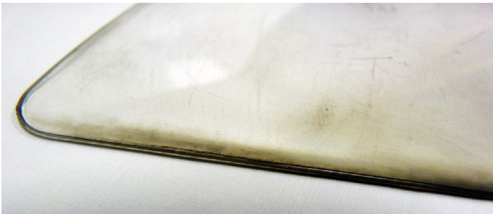
Fig. 9: 1 mm thick PETG cut with a scan head, creating discolored edges.
