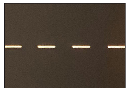
In this example the thin film was cut using a Synrad vi30+, yielding clean, consistent cuts.
