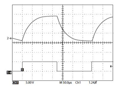
Figure 4-3 Typical optical output pulse (50%) duty cycle at 3kHz.
