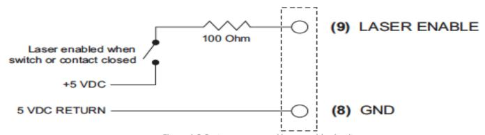
Figure 4-9 Customer powered laser enable circuit.
