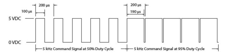
Figure 4-5 PWM Command signal waveform
