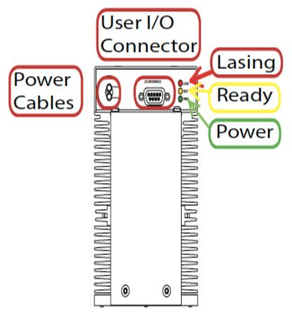
Figure 3-2 OEM vi30/40 Rear panel controls and indicators.
