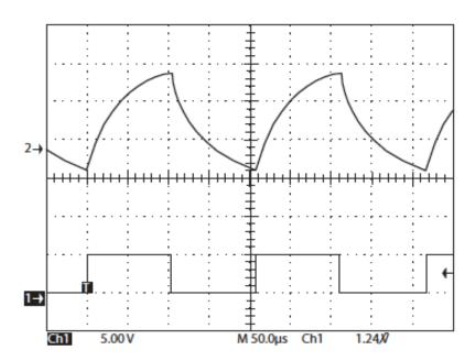
Figure 4-4 Typical optical output pulse (50%) duty cycle at 5kHz.
