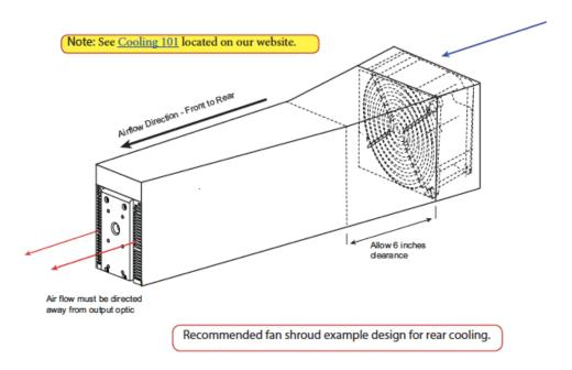
Figure 4.2 Recommended fan shroud example
