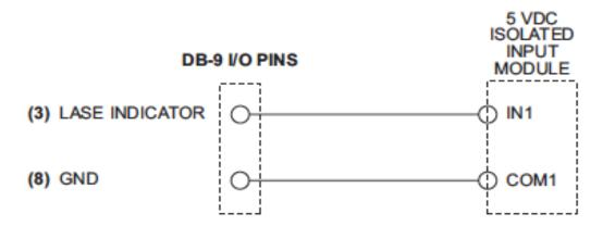
Figure 4-12 Lase indicator output to PLC input
