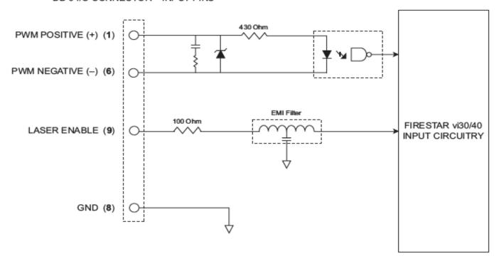
Figure 4-7 Input equivalent schematic.
