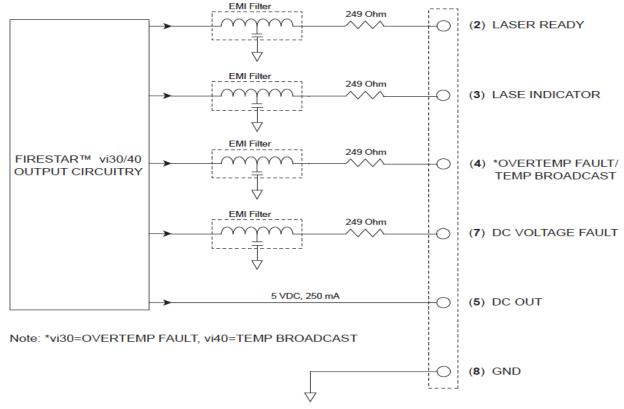
Figure 4-11 Output equivalent schematic.
