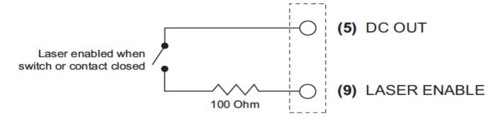
Figure 4-8 OEM vi30/40 powered Laser Enable circuit.
