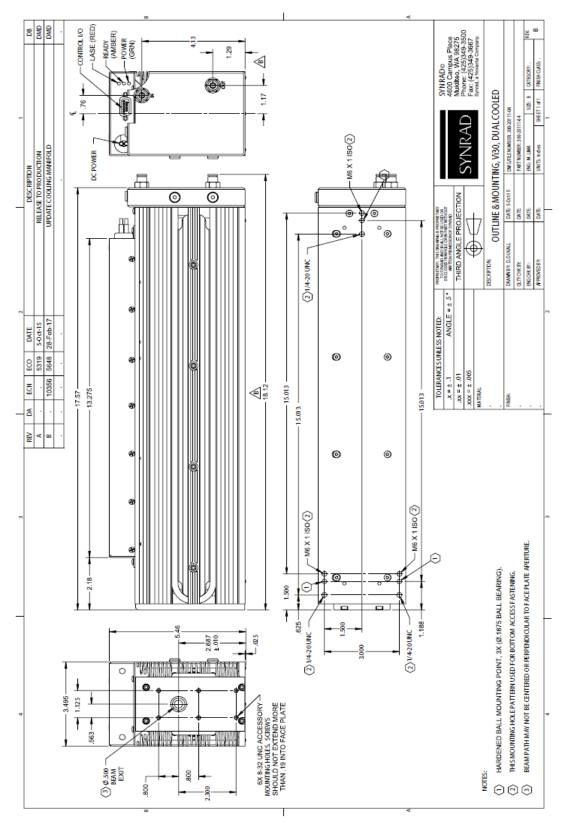
Figure 4-17 OEM vi30 Dual-cooled outline and mounting diagram
