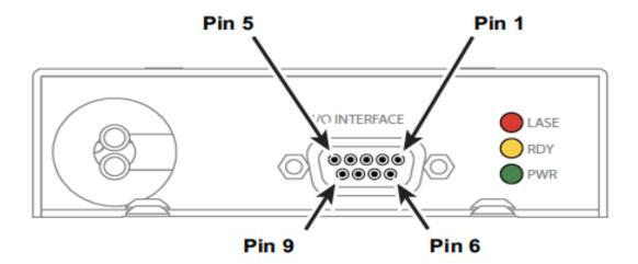
Figure 4-6 DB-9 I/O connector pinouts.
