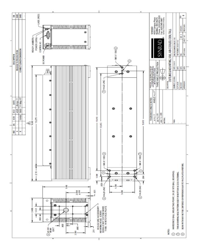
Figure 4-16 OEM vi30 package outline and mounting dimensions
