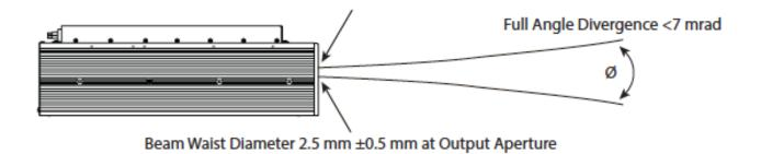
Figure 4-1 vi30/40 beam ellipticity.
