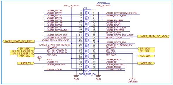
Figure 13 - Connector J18 (Laser) Pinouts
