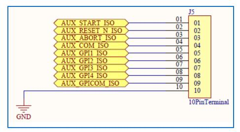
Figure 40 - J5 System Control Inputs
