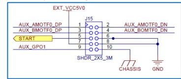
The following figure contains the pinout drawing for Connector J15 (MOTF-0)
