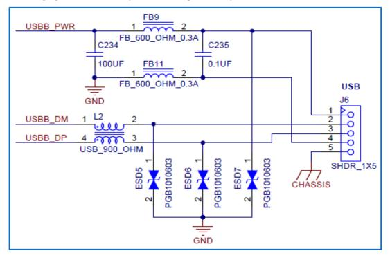
Figure 17 - Connector J6 (USB Port 2 Header) Pinouts
