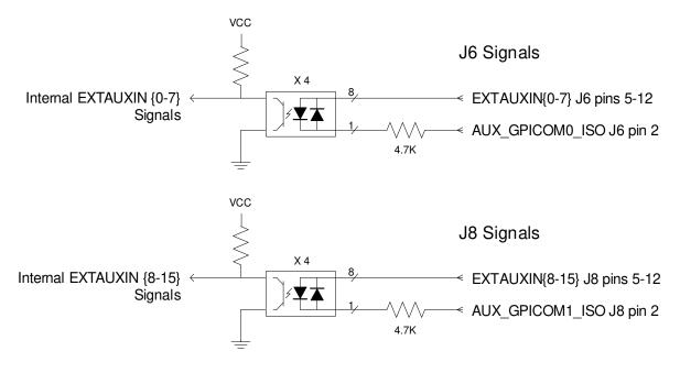
Figure 35 - Extended Inputs Signal Conditioning
