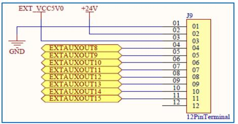
Figure 37 - J9 Extended Outputs Bank 1
