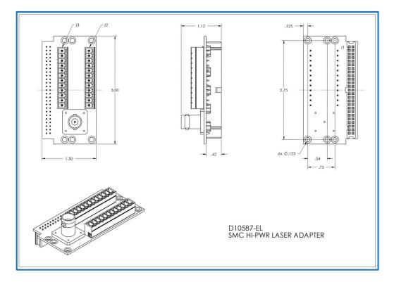
Figure 46 - High-Power laser adapter mechanical layout
