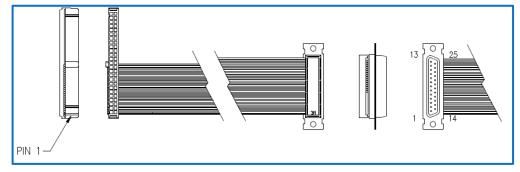
Figure 42 - IPG Laser Adapter Cable Mechanical Layout
