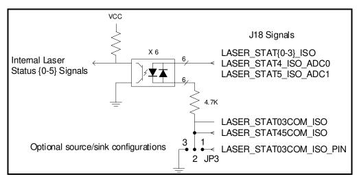
Figure 14 - LASER\_STAT Signal Conditioning
