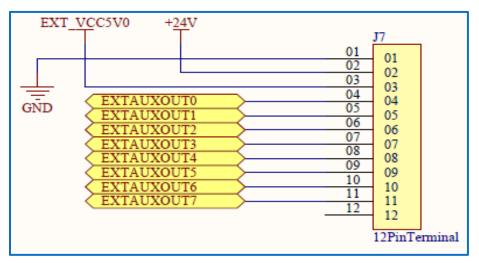
Figure 36 - J7 Extended Outputs Bank 0
