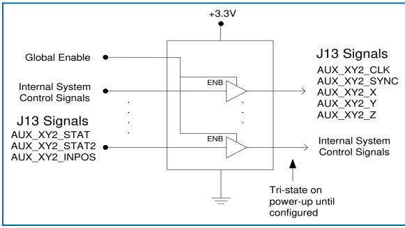
Figure 27 - Signal Conditioning for Auxiliary XY2-100 Signals (J13)
