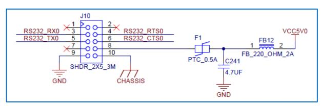
Figure 6 - Connector J10 (RS-232) Pinouts
