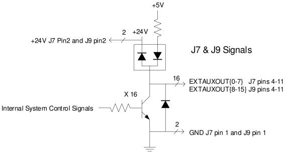
Figure 38 - Extended Outputs Signal Conditioning
