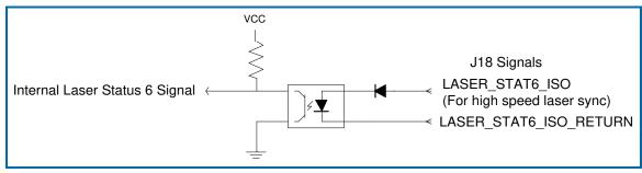
Figure 19 - Signal Conditioning for High-speed Laser Synchronization (J18)
