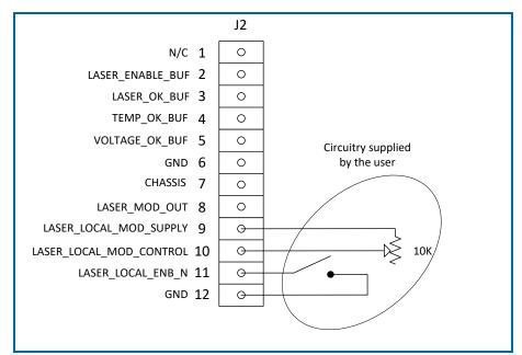
Figure 51 - Remote Modulation Control Configuration
