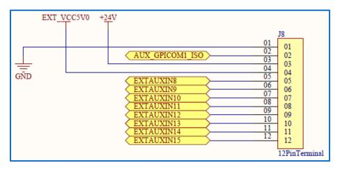
Figure 34 - J8 Extended Inputs Bank 1
