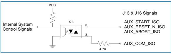
Figure 22 - Signal Conditioning for System Control Inputs (J13 and J16)
