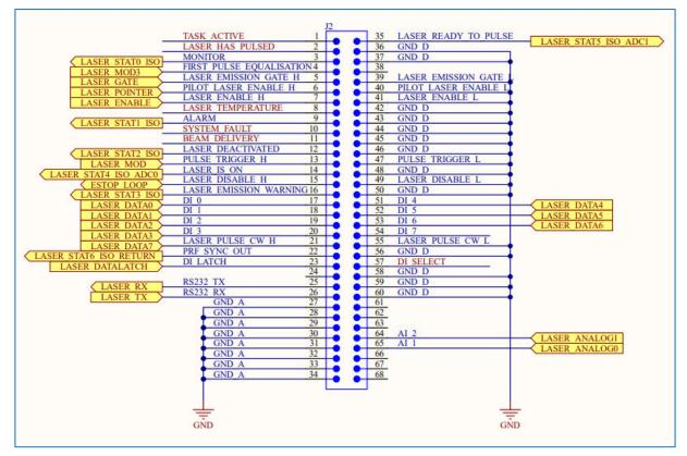
Figure 44 - SPI Laser Connector Signal Assignments
