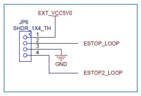
Figure 15 - Connector JP6 (E-STOP) Pinouts
