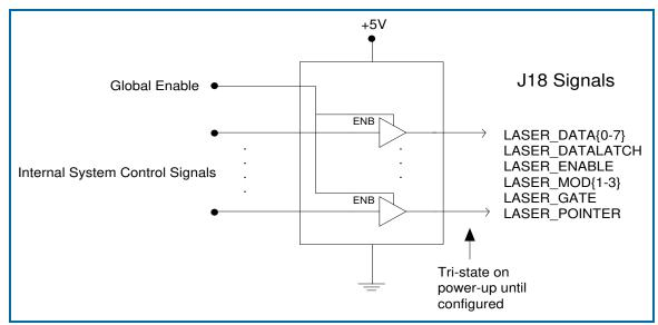
Figure 26 - Signal Conditioning for Laser Control Outputs (J18)
