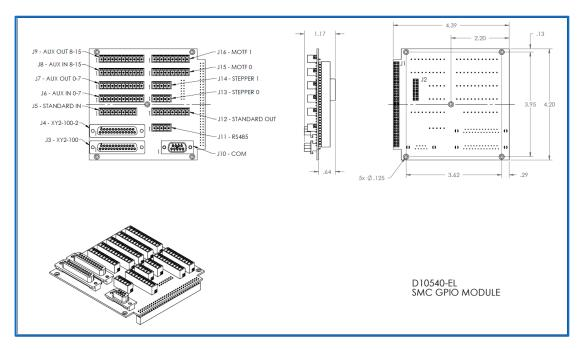
Figure 28 - Auxiliary I/O module outline drawing
