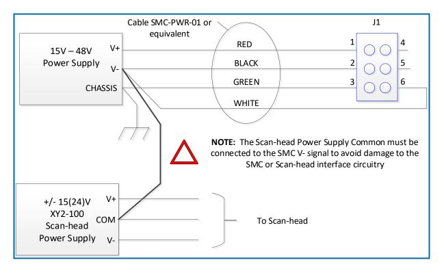
Figure 5 - Recommended Power Supply Connections
