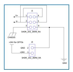
Figure 4 - Connectors J1 and J3 (Power) Pinouts
