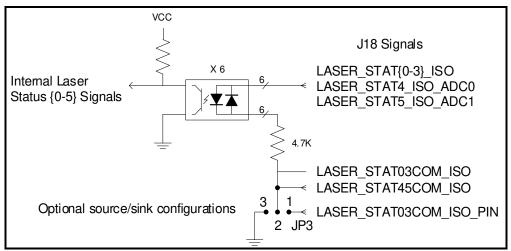
Figure 20 - Signal Conditioning for Laser Status 0-5 Signals (J18)
