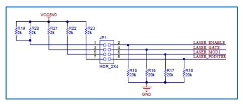
Figure 49 - Control Signal Pull-up/Pull-down Configuration
