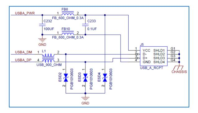
Figure 16 - Connector J5 (USB Port 1 Pinouts)
