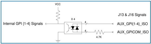
Figure 21 - Signal Conditioning for General Purpose Inputs (J13 and J16)
