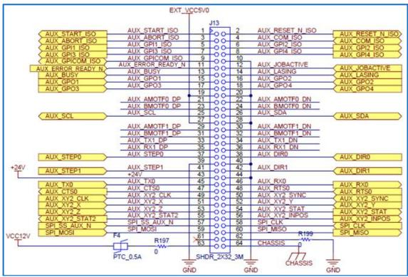
Figure 8 - Connector J13 (Auxiliary) Pinouts
