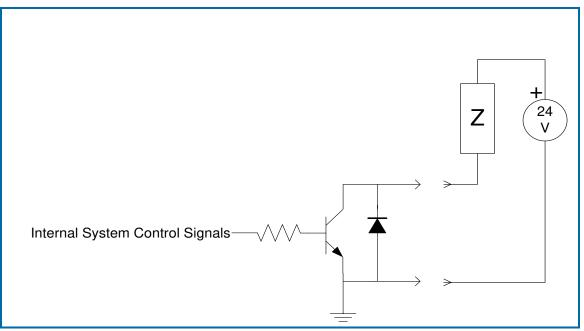
Figure 25 - Expected Usage of Digital Outputs
