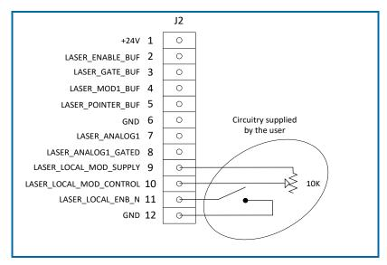
Figure 48 - Remote Modulation Control Configuration
