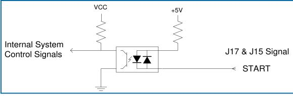
Figure 23 - Signal Conditioning for START Input (J17 and J15)
