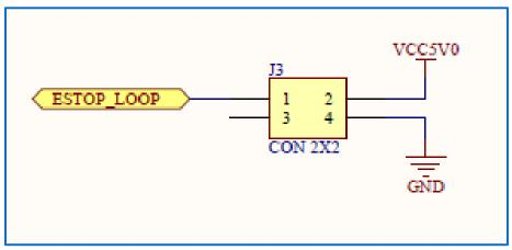
Figure 45 - E-STOP Connector Signal Assignments
