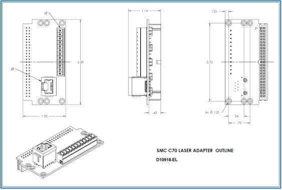
Figure 50 - Coherent C70 Laser Adapter Mechanical Layout
