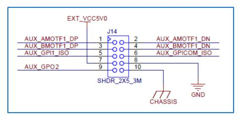
Figure 9 - Connector J14 (MOTF-1) Pinouts
