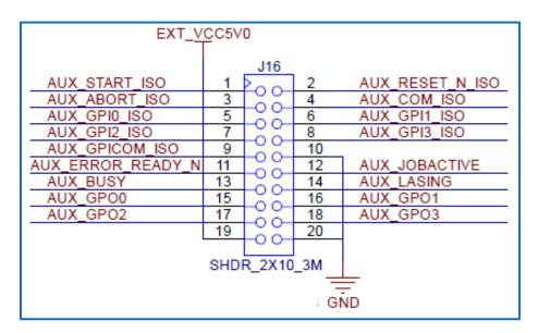
Figure 11 - Connector J16 (Control) Pinouts
