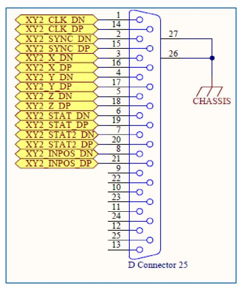
Figure 29 - J3 XY2-100 Port 1 and J4 XY2-100 Port 2
