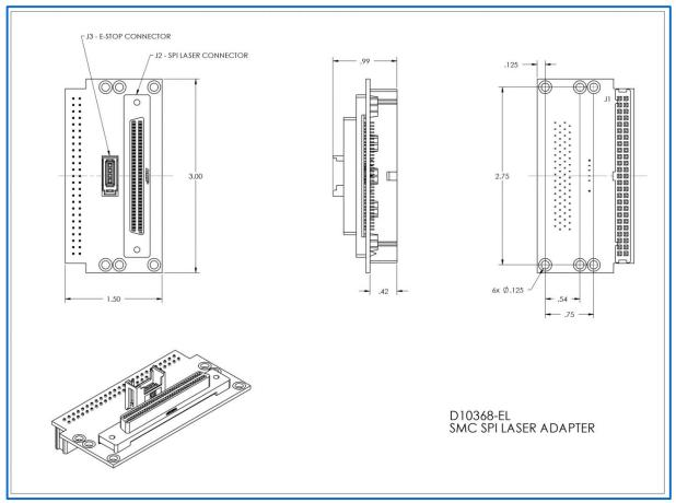
Figure 43 - SPI Laser Adapter Mechanical Layout
