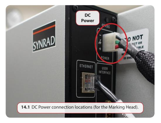
15. Connect the Laser **negative** (**black**) and the **positive** (**red**) DC power into the **laser's power** supply.
