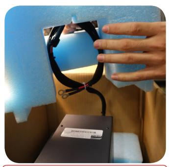
**6.1** Gently remove the foam out from under any ports sticking out of the back end of the laser. Take care not to pull the wire when seating or un-seating the foam.
