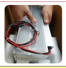
**5.2 Correct hand and hand** placement for *lifting* the laser out of the box.
