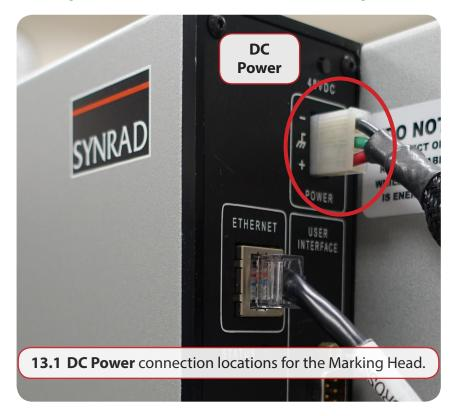
14. Connect the Laser negative (black) and the positive (red) DC power into the Laser's power supply.
