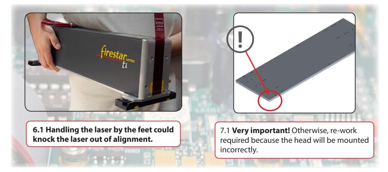
7. Remove the **rail** from the packaging. Ensure the notch is facing down and to the left.
