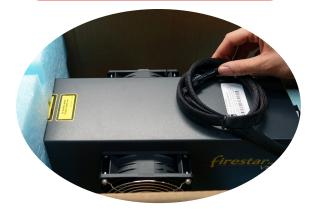
**5.2 Correct hand and wire harness** placement for *lifting* the laser out of the box.
