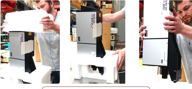
3.1 Remove and retain the marking head foam.
