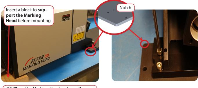
8.1 **Place** the Marking Head on the **rail as shown**, a block may be used to **support the marking head** until it is mounted to the rail.
