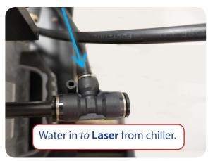
**Note:** Assure the port for water out from Marking Head is connected to the water out from Laser to chiller. Same is true for the water in from the chiller to the Marking Head/Laser.
