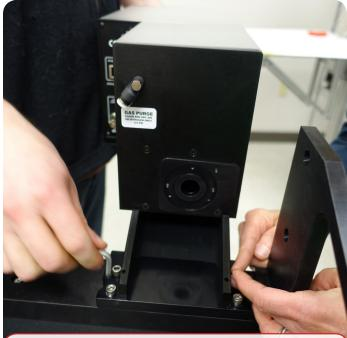
**10.1** May take two (2) people, one to hold the Marking Head onto the rail, the other to tighten four (4) mounting bolts.
