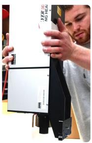
Remove protective cover after final mounting. 3.1 Remove and retain the marking head foam.
