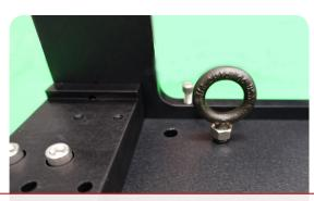
**7.4** Then place the two eyebolts with nuts onto the front end of the rail as shown.
