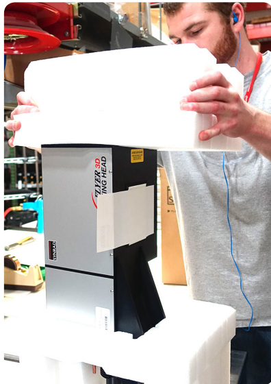
Fig 3. When removing the Marking Head from the foam, don't forget to look at the bottom of the Marking Head box for the components i.e. clamp and tube.
