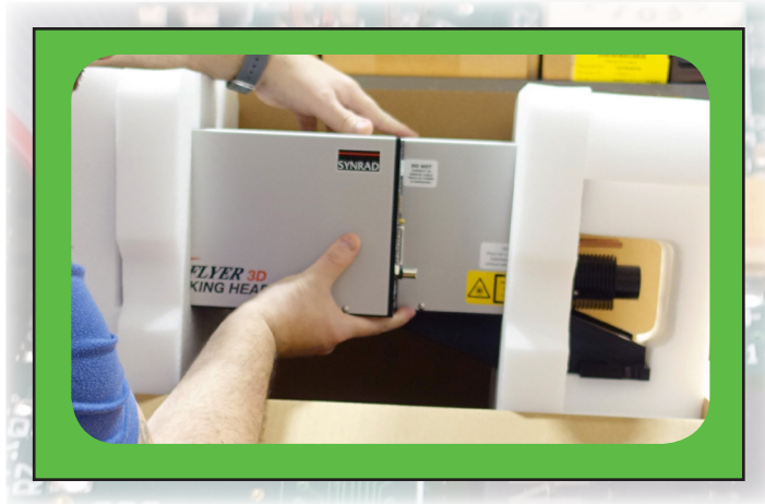
Fig 1. Lifting the Marking Head correctly by holding in the middle.
