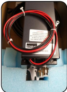
3.3. **Drrape the wire harness across the top of the laser housing** when carrying.
