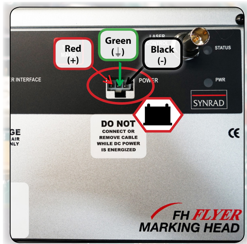
13.1 DC Power connection locations (for the Marking Head) to the power supply.
