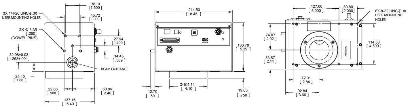
Scan head, Synrad CO<sub>2</sub> laser (10 - 150 W) and alignment fixture
