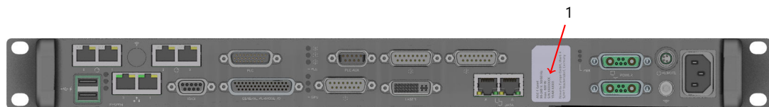
Figure 3.2.: ASC-1: Positioning of labels at the rear
