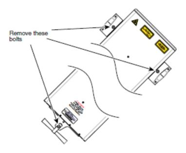
Figure 2-2 Removing lifting handles.
