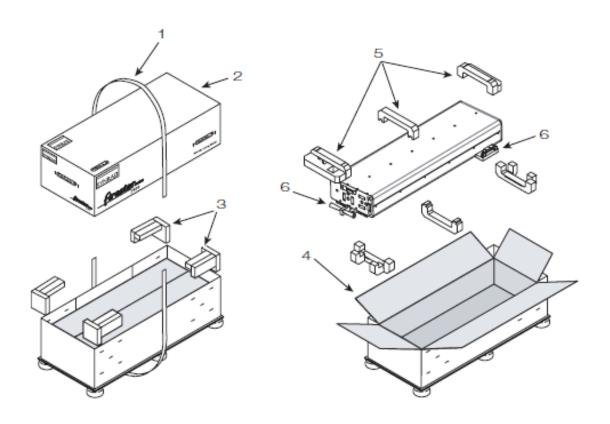
Figure 2-1 Unpacking the laser.
