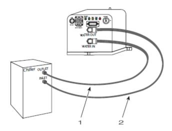
Figure 2-7 F201 cooling connections.
