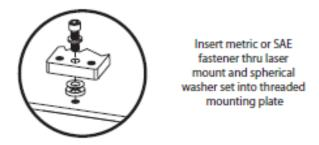
Figure 2-5 Detail of fastening into mounting surface.
