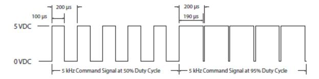
Figure 4-4 PWM Command signal waveform.
