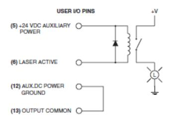
Figure 4-13 F201 laser output driving relay.
