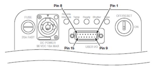
Figure 4-5 User I/O connector pinouts.
