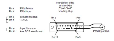
Figure 4-8 Input equivalent schematic.
