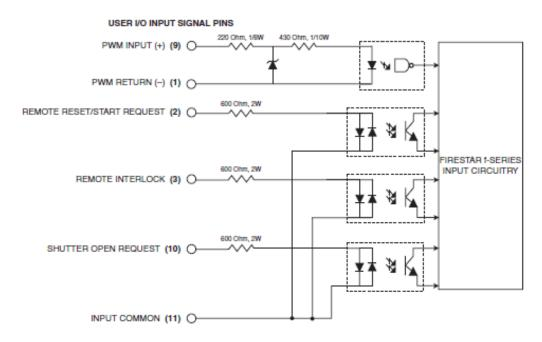
Figure 4-7 Quick Start Plug wiring diagram.
