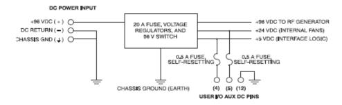
Figure 4-6 Auxiliary power supply wiring.
