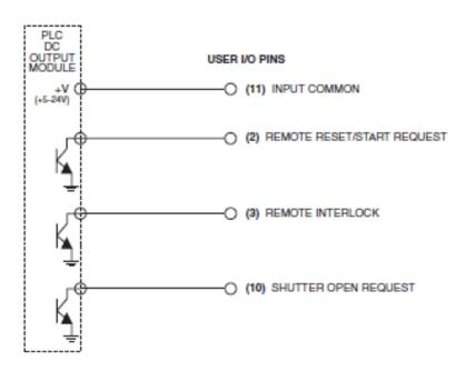
Figure 4-11 Multiple PLC driven inputs.
