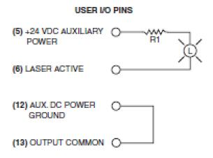
Figure 4-12 F201 laser output driving warning lamp.
