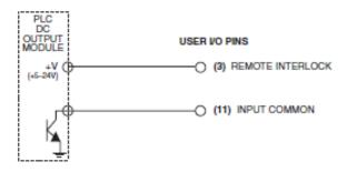
Figure 4-10 PLC driven interlock signal.
