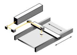
Figure 4-2 "Flying optics" beam path.
