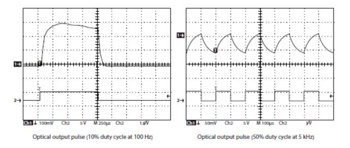
Figure 4-3 Typical F201 laser f201 waveforms.
