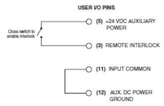
Figure 4-8 Customer-supplied interlock.
