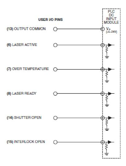
Figure 4-14 F201 laser output driving PLC input module.
