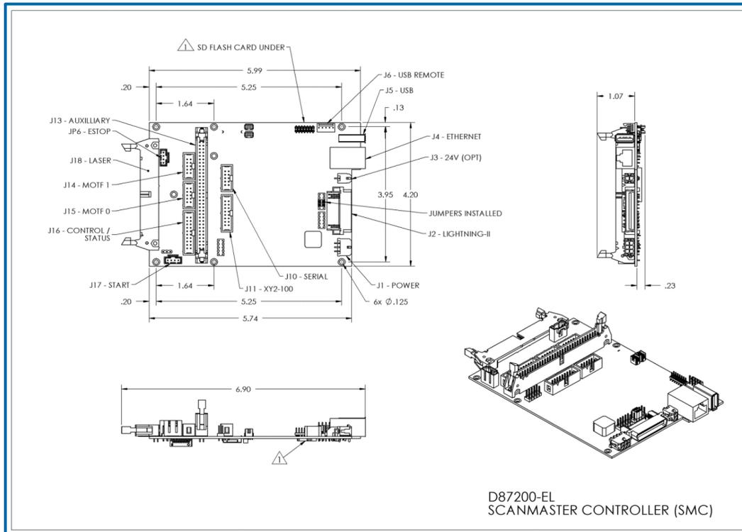
Figure 3 - SMC connector layout and dimensions
