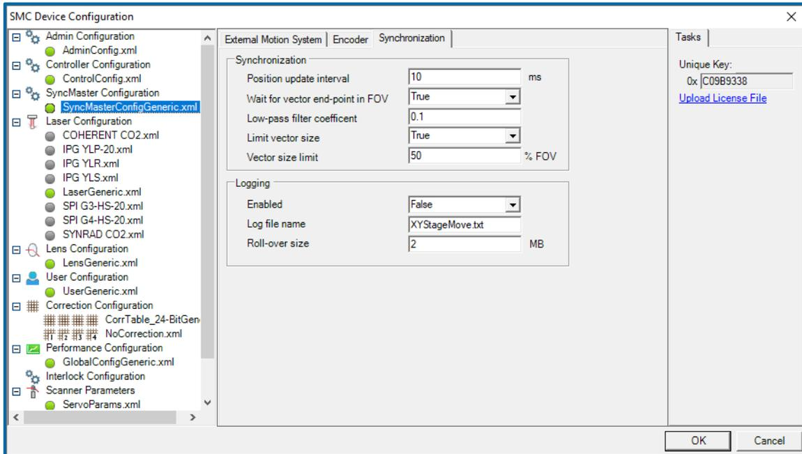
Figure 16 - SyncMaster Configuration - Synchronization
