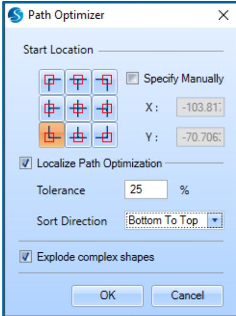
The purpose of the localized window optimization is to minimize the amount of motion the work-piece positioning system needs to do in order to keep the scan-head field of view over the appropriate location. This permits managing the motion between a heavier and slower axis versus a lighter and faster axis.
