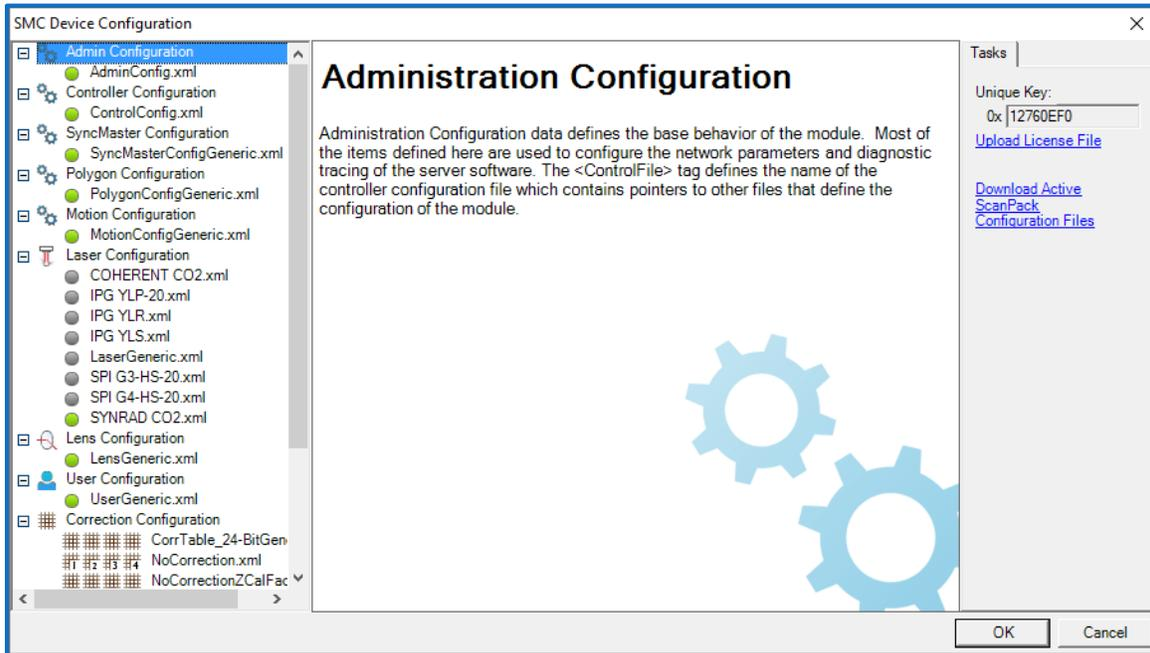
Figure 12 - SMC Device Configuration – AdminConfig
