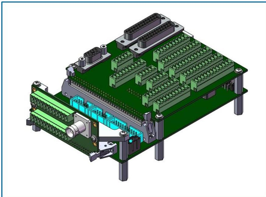
Figure 2 - SMC with laser adaptor and auxiliary I/O module
