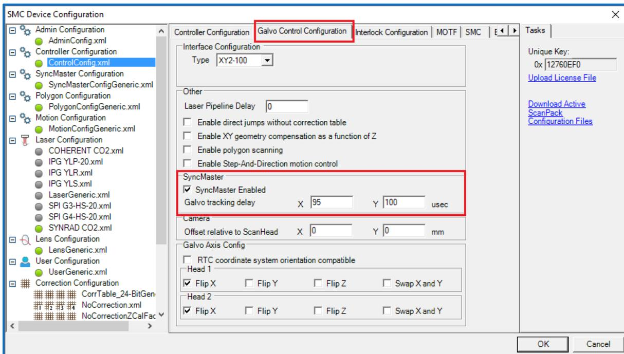
Figure 9 - SMC Device Configuration – Galvo Control Configuration
