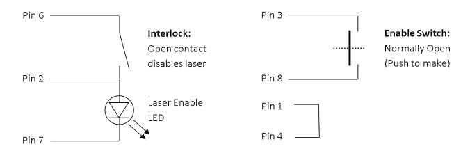
If the Interlock connection is broken or if the laser head or controller overheats, the laser will shut down. The Interlock connection must be re-made or the temperature restored to normal before the laser can be re-started.
