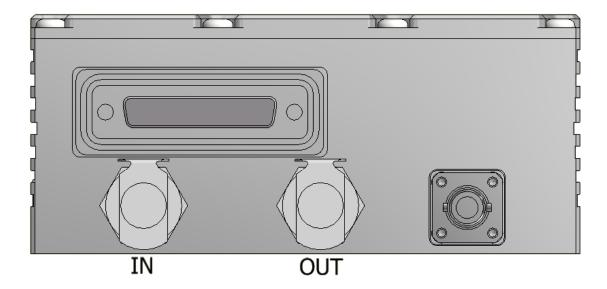
The required water connectors are standard CPC coupling inserts and a tubing size of approximately 1/4" or 3/8" is suitable.
