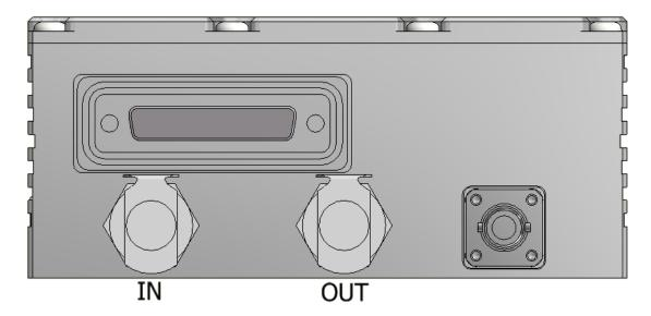
The required water connectors are standard CPC coupling inserts and a tubing size of approximately 1/4" or 3/8" is suitable. For further information on heatsinking your laser system, please consult your sales representative who may be able to provide an alternative heatsink solution if water cooling is not possible.
