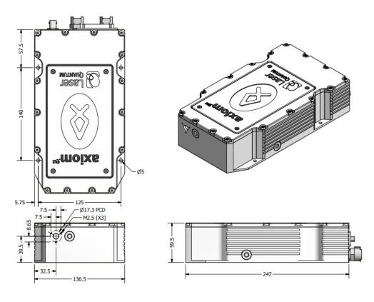
mpc32 PSU Weight: 1.6 kg
