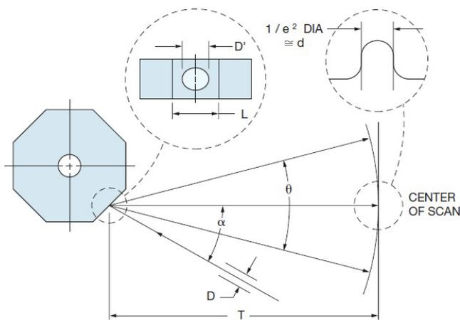
FIGURE 1: SCAN SYSTEM WITHOUT SCAN LENS
