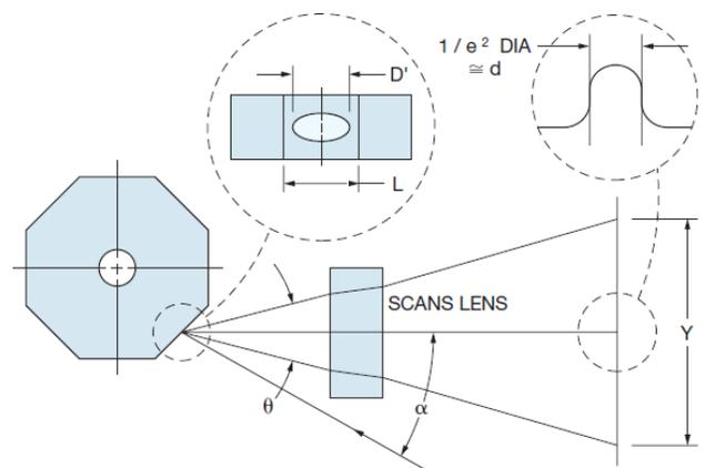
FIGURE 2: SCAN SYSTEM WITH SCAN LENS
