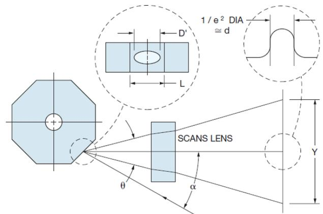
FIGURE 2: SCAN SYSTEM WITH SCAN LENS
