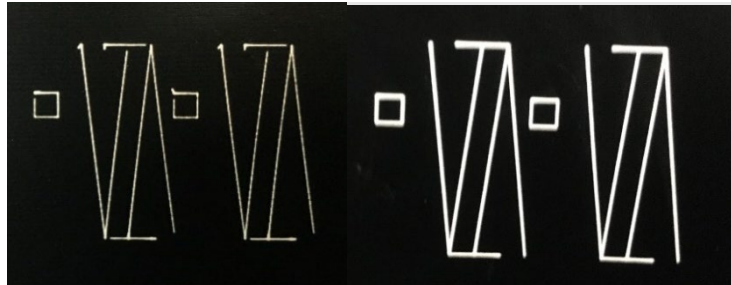
Figure 13: Example of badly adjusted delay settings (left) and well-adjusted delay settings (right)
