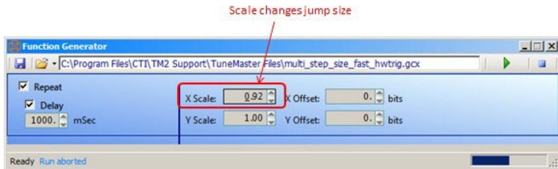
Figure 10 - Scale Command in Function Generator
