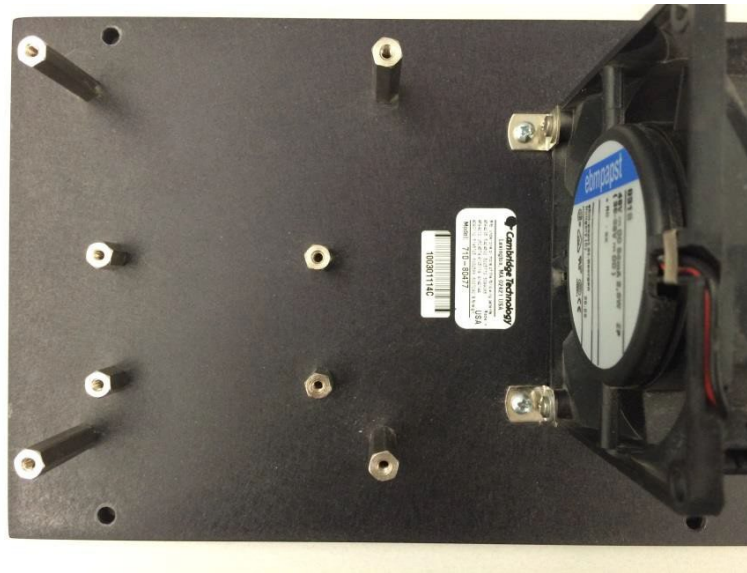
Figure 3 - Four "long" standoffs and four "short" standoffs still attached to the baseplate
