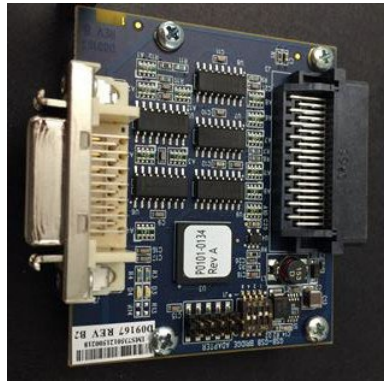
Figure 1 - The GSBUS interface board
