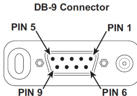
Figure 4-8 Physical layout of Series 48 DB-9 Connector.
