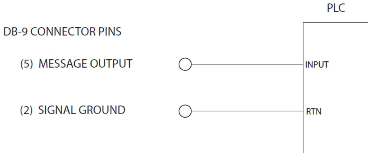
Figure 4-12 Message Output to PLC input.
