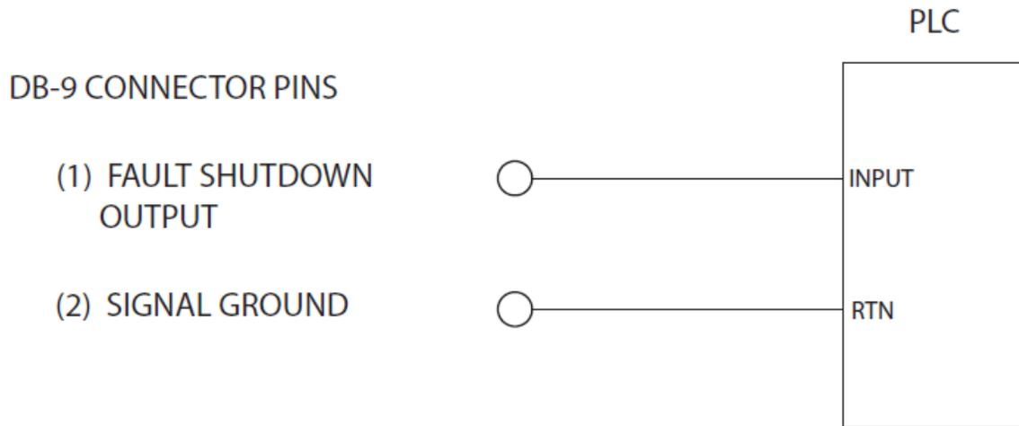
Figure 4-13 Fault Shutdown Output to PLC input.
