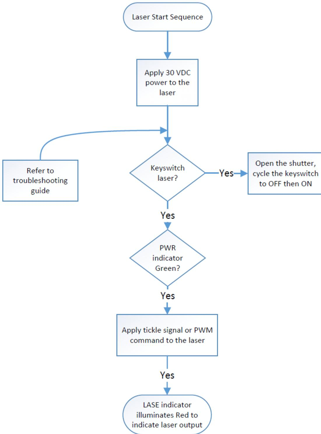
Figure 5-1 48 series operational flowchart.
