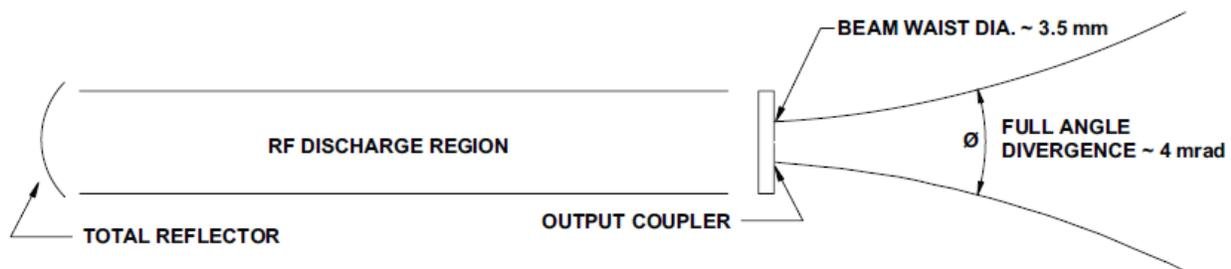
Figure 4-1 beam characteristics
