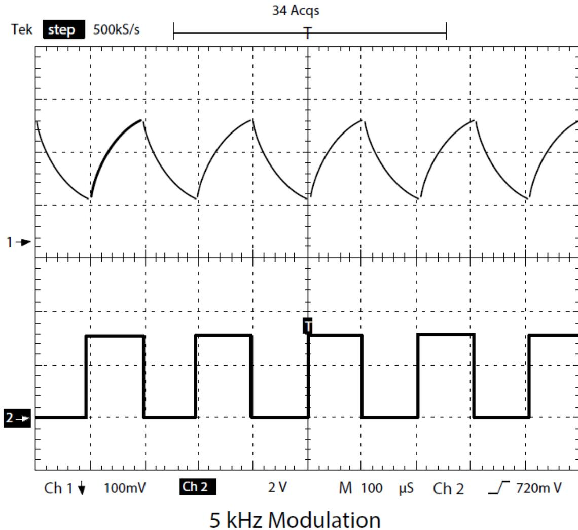
Figure 4-5 Series 48-5 kHz waveform. The upper waveform is laser output, the lower wave form is PWM input.
