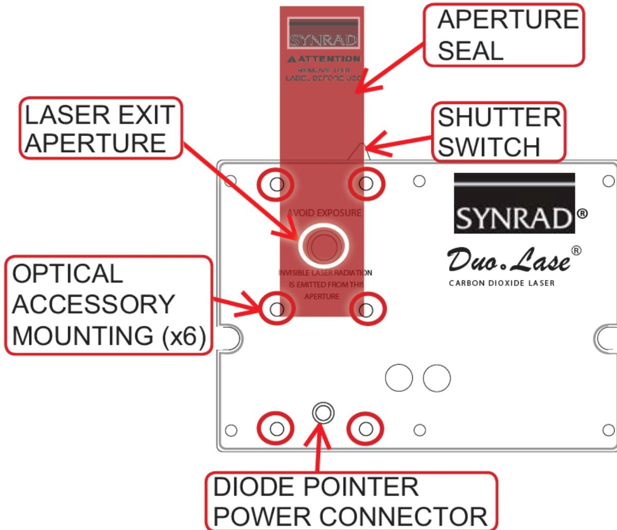
Figure 3-4 48-5 Front panel controls and indicators.
