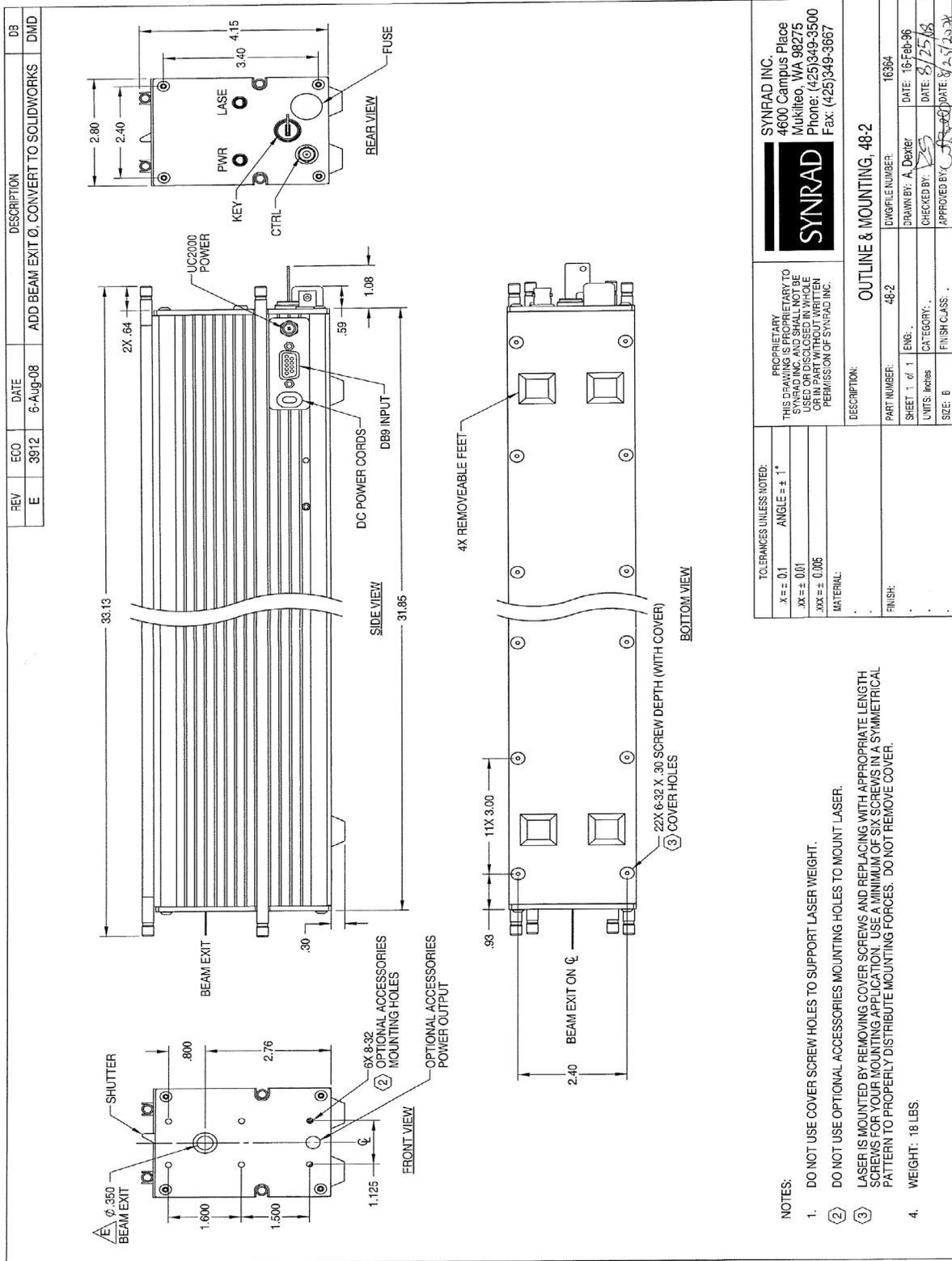
Figure 4-15 Model 48-2 package outline and mounting dimensions, 2 of 2.
